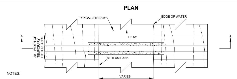
1. TRENCH PLUGS SHALL BE INSTALLED IMMEDIATELY PRIOR TO THE STREAM BANK AND 50' IN EITHER DIRECTION.
