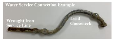
Although no longer permitted, and not installed within EWW's system since the mid-1940's, lead goosenecks are short sections of pipe (1-2 feet) that were historically used to connect wrought iron customer service lines to EWW's older cast-iron water mains. EWW believes eliminating all potential sources of lead is the best way to protect our customers.
