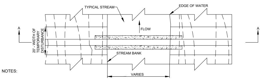
1. TRENCH PLUGS SHALL BE INSTALLED IMMEDIATELY PRIOR TO THE STREAM BANK AND 50' IN EITHER DIRECTION.
